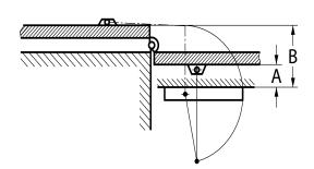
Dimension A = reveal depth Dimension B = reveal depth +2 door thickness +2 pivot point distance
