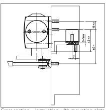
Cross section = installation with mounting plate
