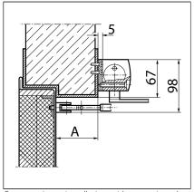
Cross section = installation with mounting pla A = max. 70 mm lintel depth with fire and smoke protection doors
