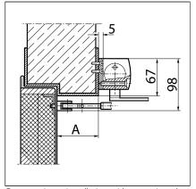
Cross section = installation with mounting plate
