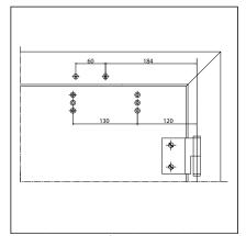
Cross section = installation with mounting plate Fitting dimensions for left-hand door
