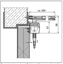
Cross section = installation with mounting plate Fitting dimensions for left-hand door
