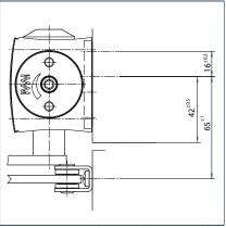
Cross section = installation with mounting plate Fitting dimensions for right-hand door
